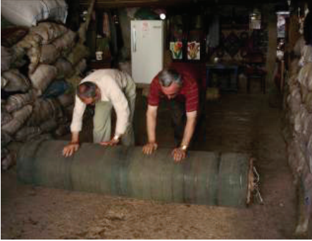
KEPENEK KALIBININ RULO YAPILMASI
